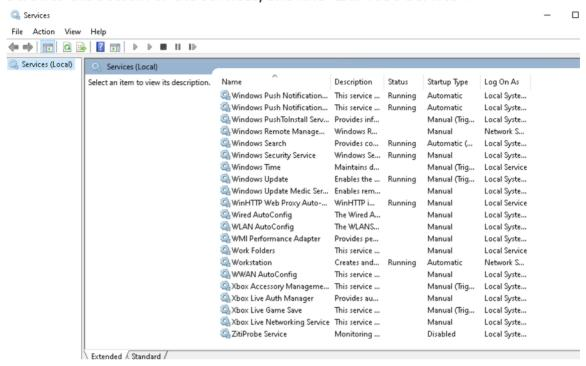
Open "ZitiProbe Service" and set the "Startup Type" to "Manual"
