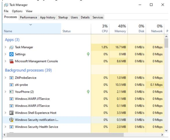
To stop the zitiprobe after data collection, you can go the "ZitiProbe Service" and press the "Stop" button
